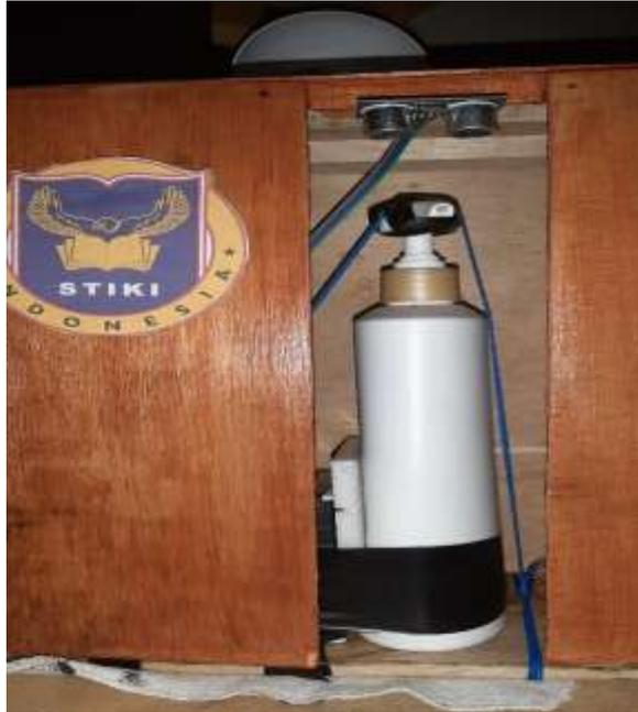
**Gambar 2.** Alat Automatic Hand Sanitizer
